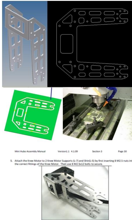
Figure 5. Key steps in manufacturing of a thigh bracket, from the CAD model and manufacturing to final assembly. [5]
